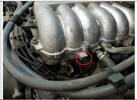
Take the shorter of the two hoses supplied with the kit, pre-install the hose clamp onto the end. This hose will run from the PCV valve to the connection on the Oil Separator closest to the intake manifold. Use the light oil to lube hose end/fitting to help with installing the hose. Tighten hose clamp, use care to not overtighten, as the PCV valve is plastic.
